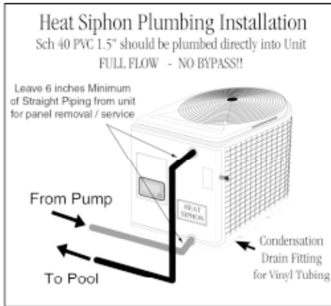
Also, plumbing shut off valves downstream of the Heat Siphon® in a way that results in the pool pump pressurizing the Heat Siphon® with no water flow can also cause short cycling damage. This is known as dead heading the pool pump.
