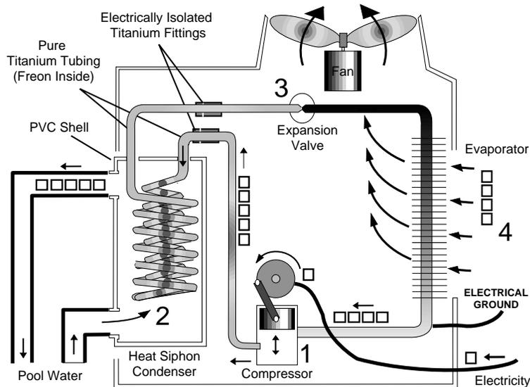
Referring to the diagram above - A unit of electrical energy (you pay for) goes into the compressor motor (1). The compressor turns this into mechanical energy and sucks cool gas from a gas-liquid freon mixture in the evaporator tubes. As the freon evaporates it absorbs four units of "free" heat from the warmer air that the fan pulls over the outside of the evaporator tubes.
